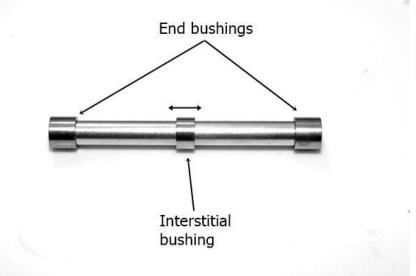
5] If all 4 rings are being used the combined length of all the blanks must be 76mm
