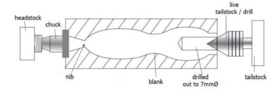
5] The handle can be sanded and finished and then removed from the lathe by cutting the nib and finishing by hand.
