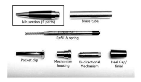
You will require a blank at least 56mm long drilled out to 10.7mm. Once the brass tube has been glued into the drilled blank, it can be turned using a bushing set either on a mandrel or between centres as you prefer.
