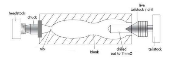
5] The handle can be sanded and finished and then removed from the lathe by cutting the nib and finishing by hand.
