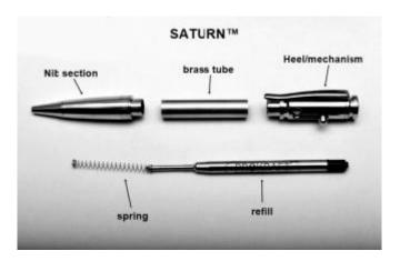
You will require a blank at least 45mm long, drilled out to 9.5mm and trimmed level with the brass tube. Once the brass tube has been glued into the drilled blank and trimmed, it can be turned using a bushing set either on a mandrel or between centres as you prefer.
